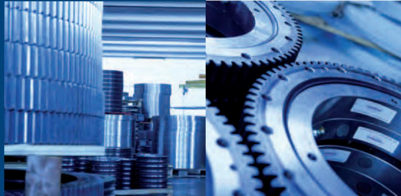
Once installed, those references are not necessarily readily available as the slewing ring might be protected by a carter or painted. In order to keep track of the serial number of the installed components it is therefore advisable to report it on the machine logbook.
